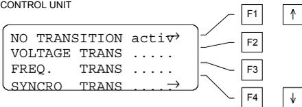
This page displays the functions which can be varied during a test.
