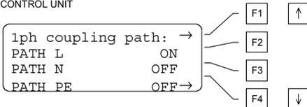
By selecting all three modes to ON the paths will be switched successively after test time has expired. *Single phase coupling menu*
