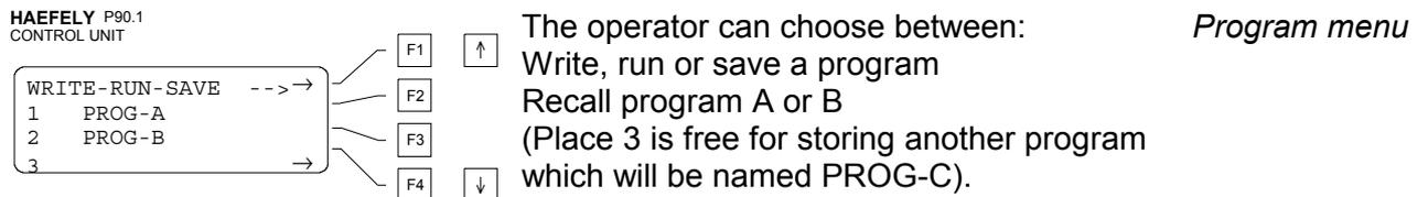
If a program has been saved to memory (ex PROG-A), it is easy to recall simply by pressing the corresponding key (ex F2). The program can then be run by pressing START / STOP.
